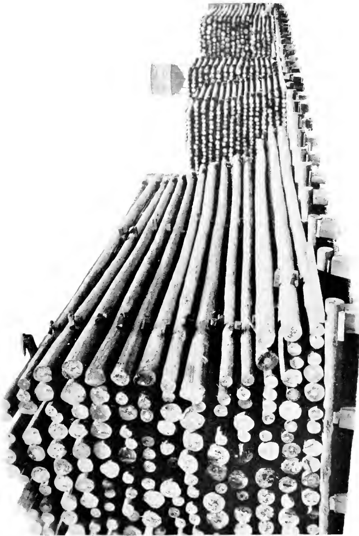
Well-piled poles in an air-seasoning yard. Each pile is high above the ground on treated piers and stringers. Heavy stickers, also treated with preservative, separate successive layers. The sanitation is excellent
